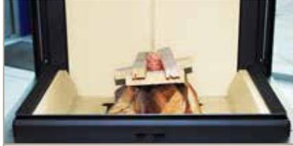
Place three logs on the chamber floor.
