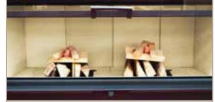
Place four logs on each ash grate on the chamber floor.
